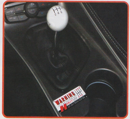
It wouldn't be a real Hurst Heritage by GSS without a Hurst shifter. This 40th Anniversary Edition is equipped with a Hurst Billet Plus Short Throw Shifter. Ronnie Sox would have been right at home in this Hemi 'Cuda bangin' all six gears.
