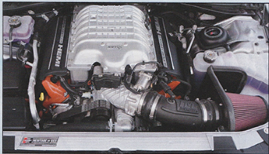
Supercharged Hemi is enhanced with Flowmaster Delta Force cold air intake.
