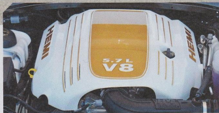
Painted engine cover is one of the few options in the 300 H package. Flowmaster Delta Force cold air intake is a standard upgrade.
