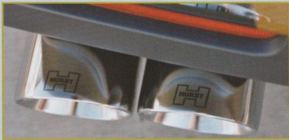
The Pro Stock inspired 16 plug Hemi heads exhale through an ultra-low restriction Flowmaster Outlaw cat back dual exhaust system that's capped off with a quartet of 4-inch double wall Hurst logo exhaust tips.
