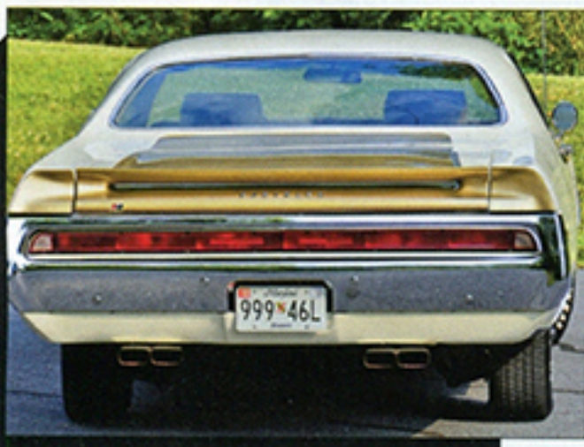
The decklid, like the hood, was fiberglass, with a molded spoiler and a Hurst emblem.
