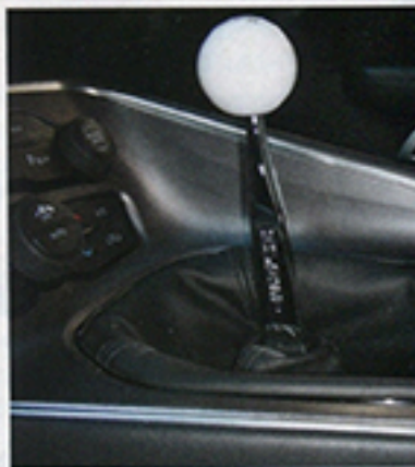
Since the Challenger was equipped with a six-speed manual transmission, it just wouldn't be a Hurst without a Hurst shifter.
