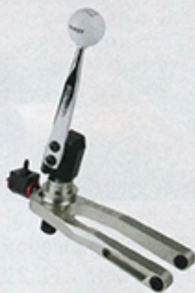
Since the Challenger was equipped with a six-speed manual transmission, it just wouldn't be a Hurst without a Hurst shifter.
